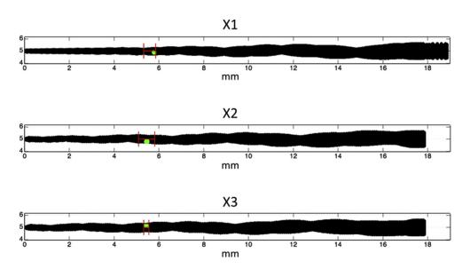
**Figure 3.** Comparison between FEA and experimental failure locations; vertical red lines denote 95% confidence intervals for the experimental failure locations, and highlighted green points denote the location of the element with the smallest NCF.
