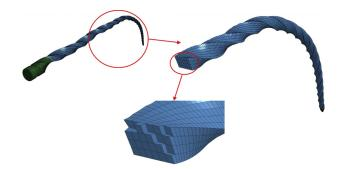
Figure 2. Finite element model of the PTN X1 file.
